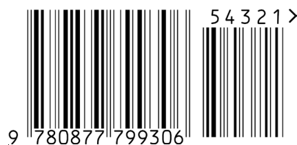
Figure 5.2.2.5.2-2. EAN-13 barcode with five-digit add-on symbol
