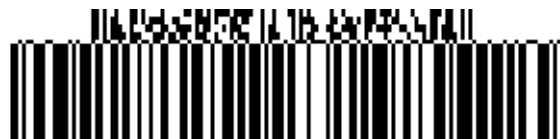
Figure 5.11.8-9. GS1-128 symbol with a four-column CC-A
