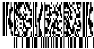
Figure 5.11.8-7. GS1 DataBar Limited symbol with a three-column CC-B
