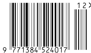
Figure 5.2.2.5.1-2. EAN-13 barcode with two-digit add-on symbol
