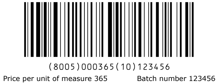
Figure 7.8.6.2-2. Data encoded in one concatenated GS1-128 symbol
