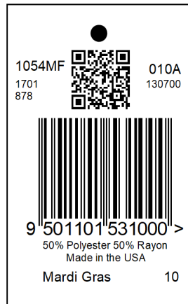
Figure 6.3.3.1-4. Maximum POS X-dimension 2D barcode placement in relation to the linear barcode example
