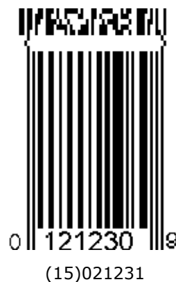
Figure 5.11.8-4. UPC-E symbol with a two-column CC-A
