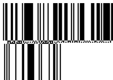
Figure 5.5.2.3.2-1. GS1 DataBar Expanded Stacked barcode
