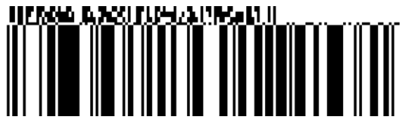
Figure 5.11.8-8. GS1 DataBar Expanded symbol with a four-column CC-A
