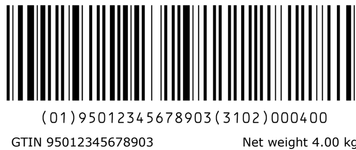
Figure 7.8.6.1-2. Data encoded in one concatenated GS1-128 symbol
