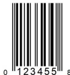
Figure 5.2.2.4-1. UPC-E barcode (encoding 012345000058 by zero-suppression)
