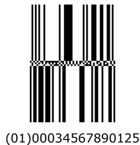
Figure 5.5.2.1.4-1. GS1 DataBar Stacked Omnidirectional barcode
