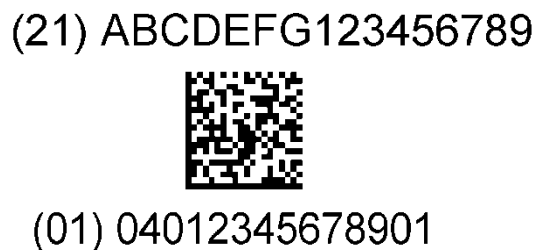
Figure 2.6.14-4. Example of GS1 DataMatrix symbol encoded with GTIN and serial number AI (21)
