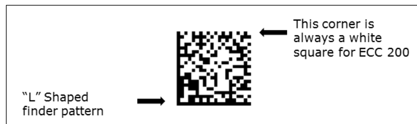
Figure 5.6.2-1. GS1 DataMatrix symbol
