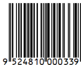
Figure 4.14-5. Example of EAN-13 with EAN/UPC HRI format
