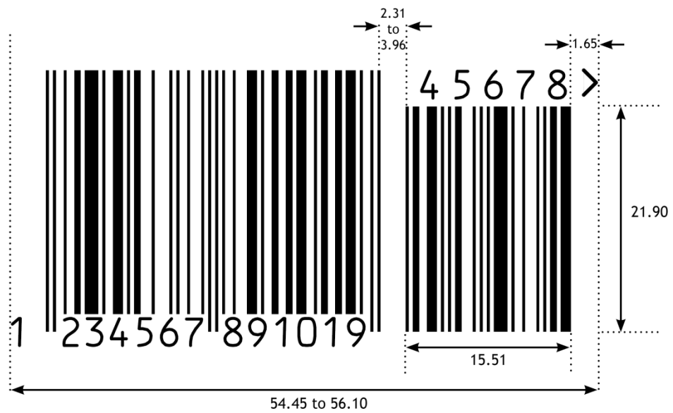
Figure 5.2.6.6-6. EAN-13 barcode with five-digit add-on symbol
