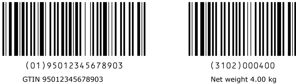
Figure 7.8.6.1-2. Data encoded in one concatenated GS1-128 symbol
