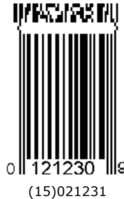
Figure 7.8.6.3-2. Example of mixed GS1 symbologies (GTIN encoded in UPC-E, Best before date in Composite)
