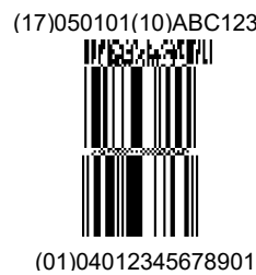
Figure 5.1.1-5. GS1 DataBar Stacked Omnidirectional barcode with a Composite Component
