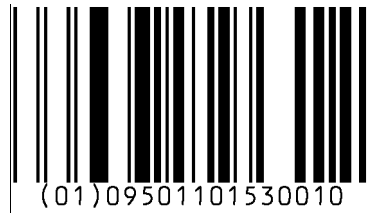
Figure 5.1.1-4. GS1 DataBar Omnidirectional barcode
