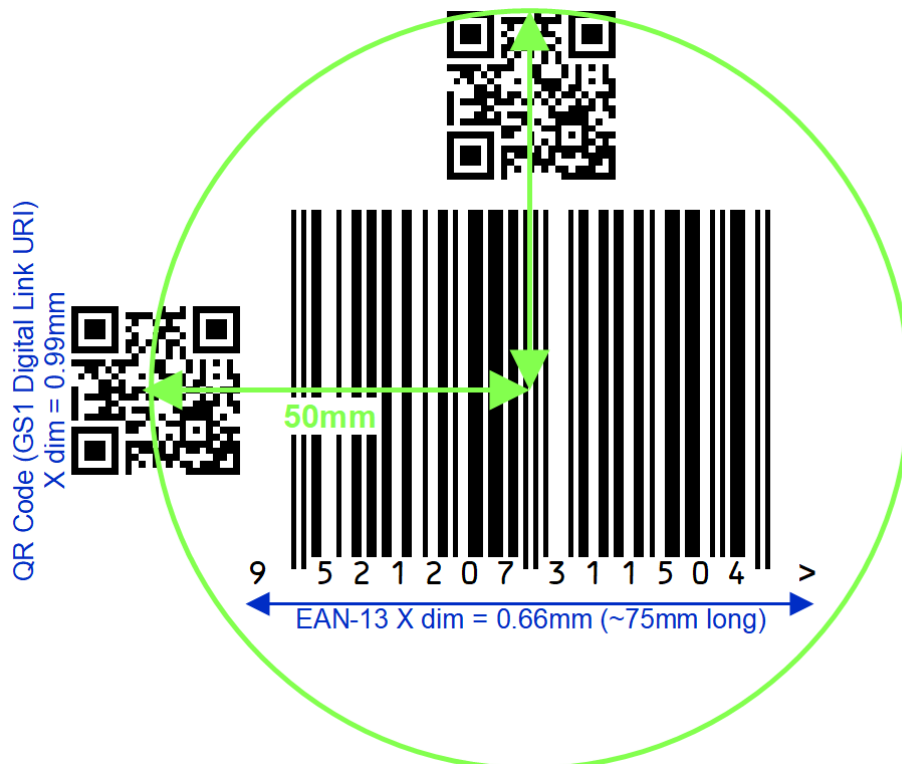
Figure 6.3.3.1-4. Maximum POS X-dimension 2D barcode placement in relation to the linear barcode example
